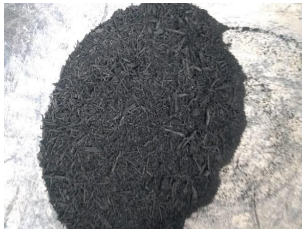
Fig.1 WTR used in the production of concrete
