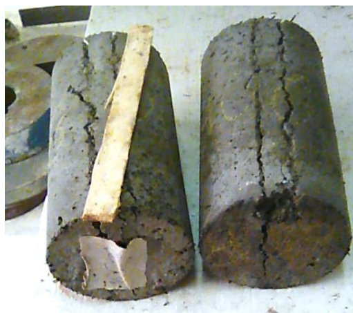
Fig.6 Cracks in the specimen for concrete with 20% incorporated content
